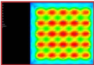
> Great for higher ceilings. Best used for fixtures mounted 30+ feet up. (This image captures a 25 foot mounting height).
