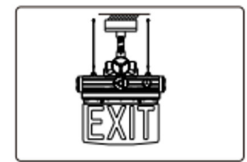
4. Install the fixture to junction box. Wiring the cable as white to L, black to N, green to G.
